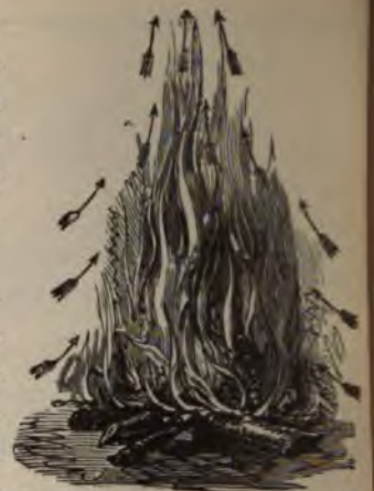
Showing the air movements created by building a fire in the open air. A strong current of cold air sets in toward the fire and the heated air rises and flows outward in every direction. Extensive fires, like the burning of Moscow and Chicago, have been followed by furious tornados.
